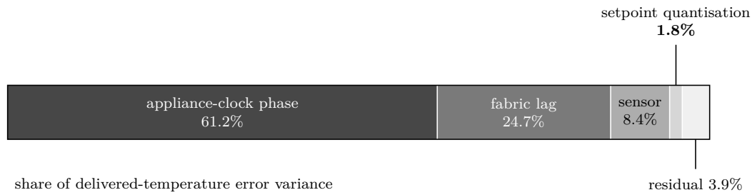
Figure 5: The bottleneck profile. Variance shares of delivered-temperature error; setpoint quantisation is 1.8%.
